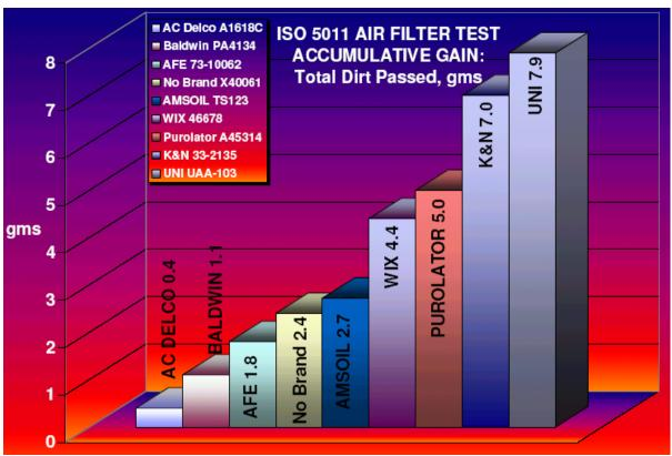
(Note: The Purolator was reported to have a seal malfunction during the test and passed more dirt than it would have with a good seal.)
