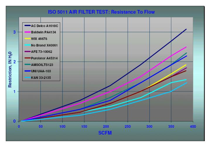
The Flow Restriction response curves for each filter have the same basic shape. However, note how the AC Filter, which passed the smallest amount of dirt and had the highest dirt capacity and efficiency, also had the highest relative restriction to flow. The less efficient filters correspondingly had less restriction to flow. This illustrates the apparent trade-offs between optimizing a filter for dirt capturing ability and maximum airflow.
