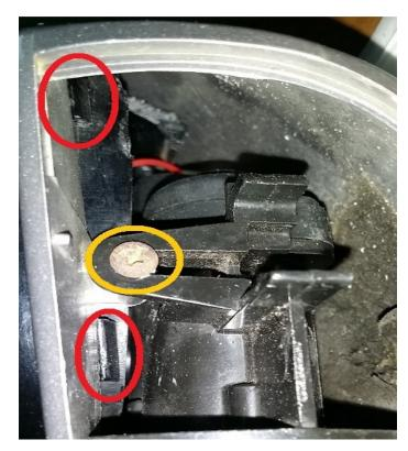
Next, you will need to heat the tip of a Cutter or a flat head screwdriver and remove a part of the black ring to free it from the housing:
