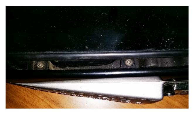
You squeeze a screwdriver in there and you start removing them one by one, VERY gently and without breaking the mirror. Note that you need to actually remove them entirely OUT of the assembly.
