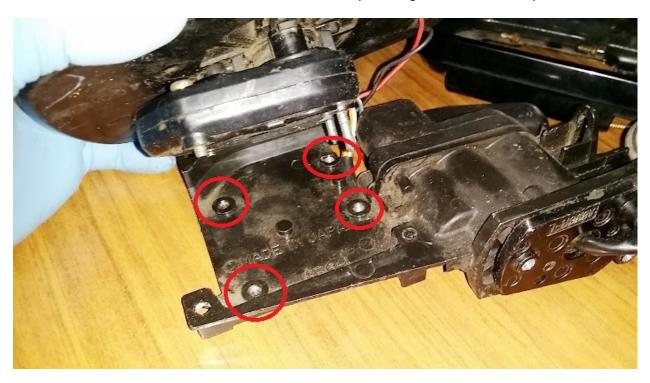
There are 4 distinct screws, (of which the ones on the right in the upper picture) need to be replaced by taller ones. You can squeeze there at most 7mm taller screws instead of the original ones, which is more than enough for the modification.
