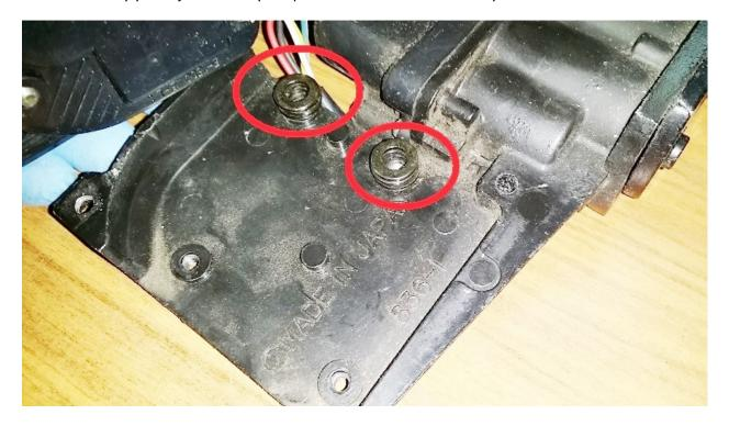
After reinstalling the mirror to its chassis, do NOT overs tighten the 4 screws till the very end or else you will risk squeezing the inner motors and rotating parts; It will become stuck. Test it out as it is on the car BEFORE putting everything back together.
