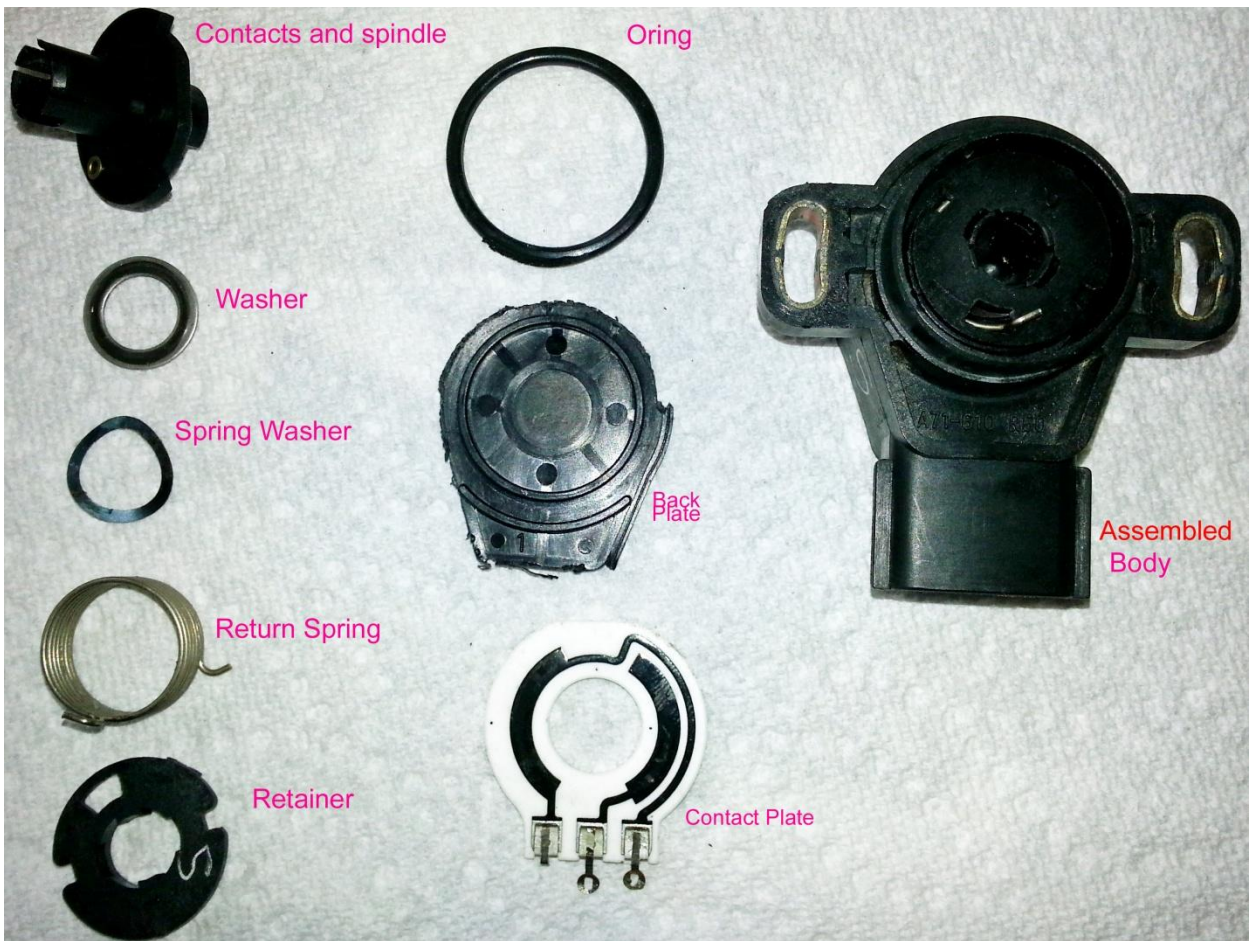
All parts. (Note the eyelet we broke on the bad SVX contact plate). The assembled view is of the Impreza TPS. On that TPS the spring hook is on the lower part of the retainer.
